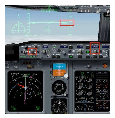
Set the altitude target to 4000, not clicking any buttons as before, when the altitude nears 19000. This simulates a clearance from ATC to descend further.
