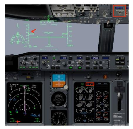
When entering the clouds turn Wing Anti-Ice ON. Keep setting slower speeds down to 200 kt. The TOR DME is now counting upwards since it's behind us.
