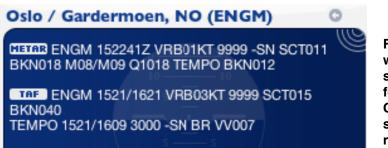
For this tutorial set the weather to 5kt wind from 11° and visibility to CAT3, standard air pressure. (The ILS is valid for CAT2 only in reality but CAT3 is used here since X-Plane isn't simulating ILS inaccuracies.) Check that runways are set as clean and dry.
