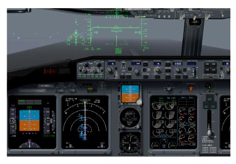
Apply Reverse thrust on touchdown. Always at least Idle power (just open the reversers without moving the throttles).
