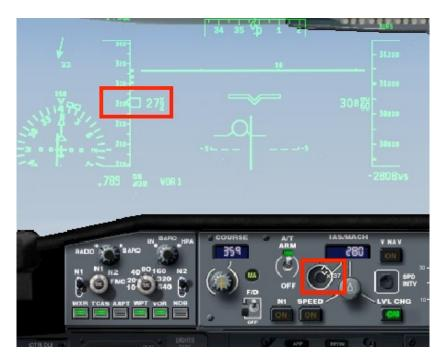
Be ready to switch to IAS speed mode when the KIAS nears 280 kt on the speedtape. Click the changeover button and set speed to 280.
