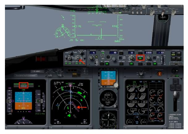
When the plane turns inbound on the Localiser and the Glideslope needle activates, arm the APP mode. Set speed to 160, drop Gear and set Flaps 25 (one click down from Flaps 15).
