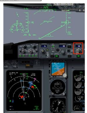
Speed must be minimum 160 kt until 4 DME on the ILS. 3000 ft is recommended for glideslope intercept. The approach has to be terminated at 102 ft radar altitude if the runway lights cannot be seen at that height.
