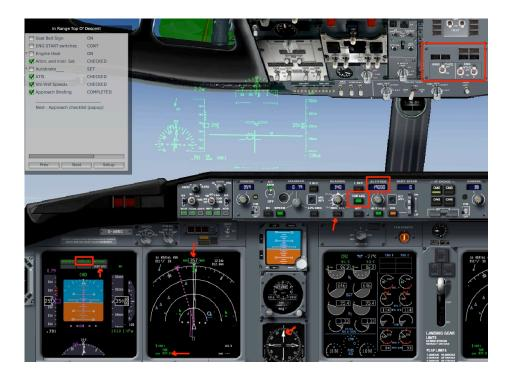
Click LVL CHG to start the descent at 80 to 70 nm DME. Set Autobrake to 2 or 3 and the start switches to CONT. Set Engine Anti-Ice to ON. Prepare for the next turn by setting heading 14° without clicking the HDG button.
