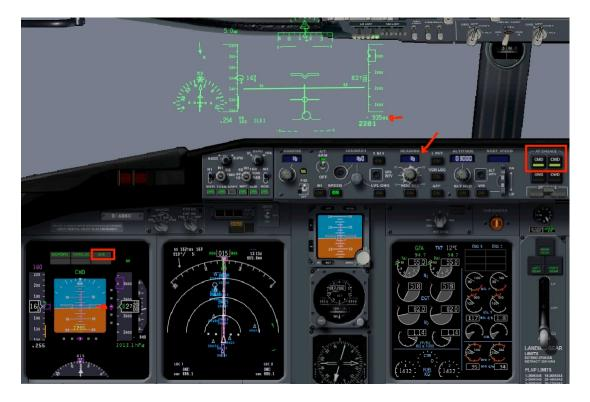
Passing DME 4.0 set Vref plus gust speed (139+5=144). Set Flaps 40. Watch the radar altimeter. Flare mode armed automatically.
